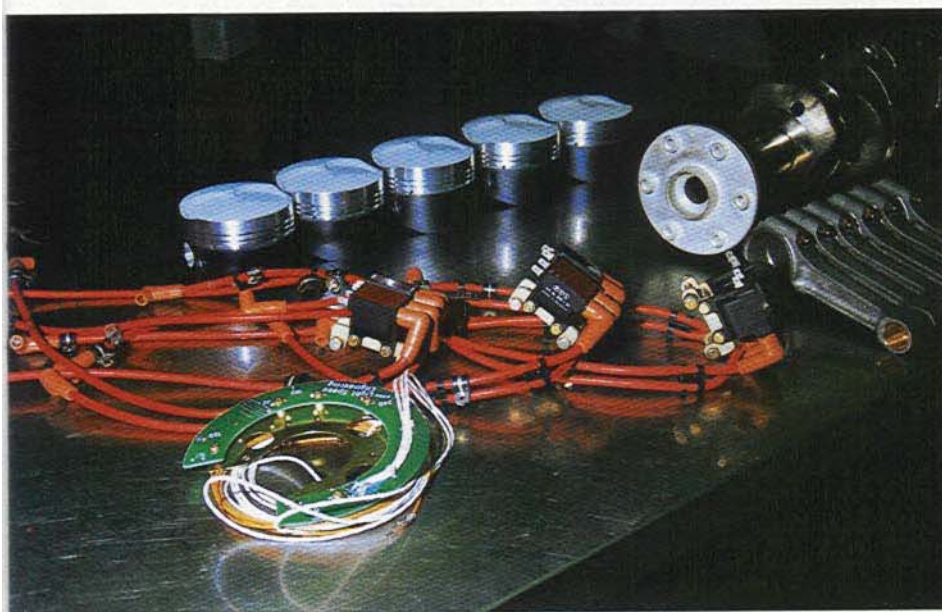
The new engine will have dual electronic ignition systems or one electronic system and one magneto.
