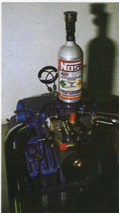
For that extra boost, like when the enemy is on your tail, nitrous can be injected through a specially designed fitting.
