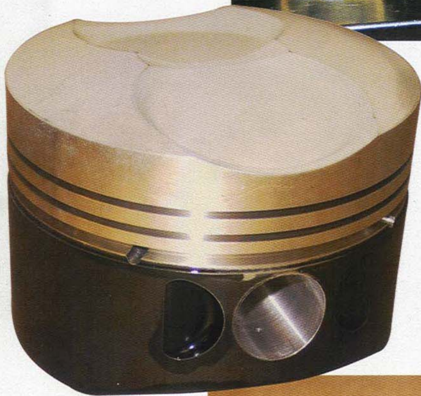
The pistons are custom made for a 10:1 compression ratio. They have a ceramic coating on top for heat resistance and a P2 Moly coating on the skirt for abrasion resistance.
