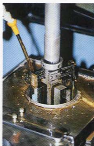
LEFT: The piston from cylinder #4 showing signs of oil bypassing the rings. RIGHT: A cylinder undergoing porting and polishing.
